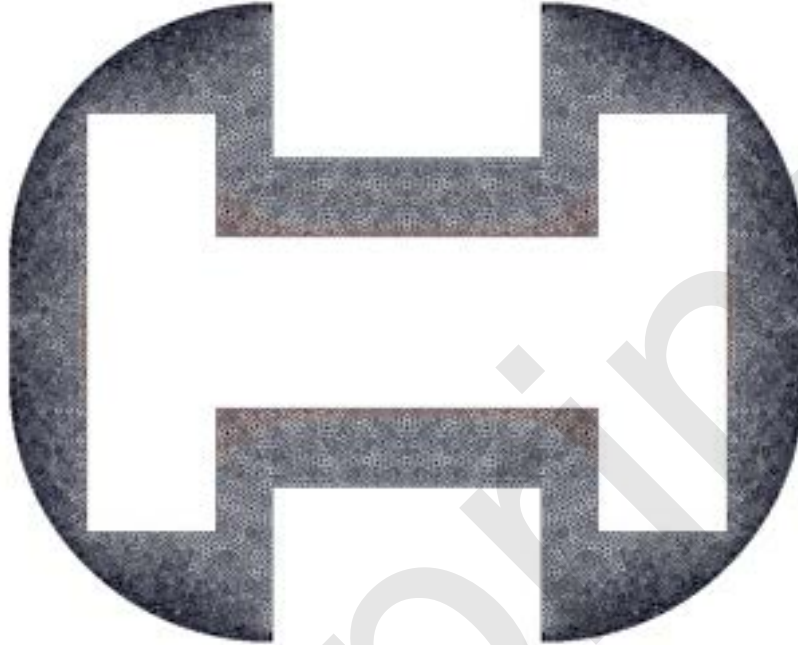
Figure 6: Triangulation of 26 184 vertices and 30 888 elements, for the cross section B-B' of the CIDR device.
